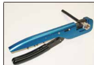
Fold braid over connector and crimp
