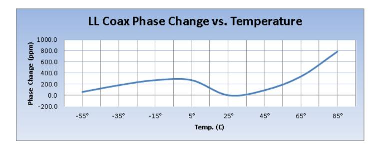
WE created the above graph by measuring the time delay change of a 10ft length of LL Low Loss coax when subjected to the following conditions:
