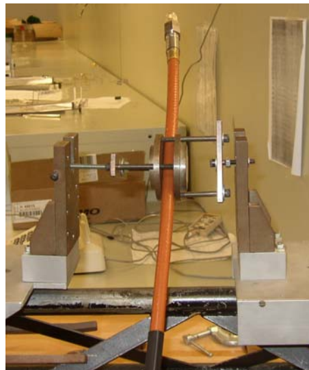
Figure 5 – Concentrated Load Test Fixture
