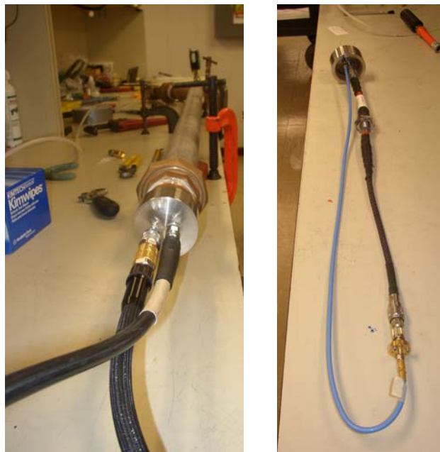
Figure 12 – Pressure setup and Cable with Test Leads
