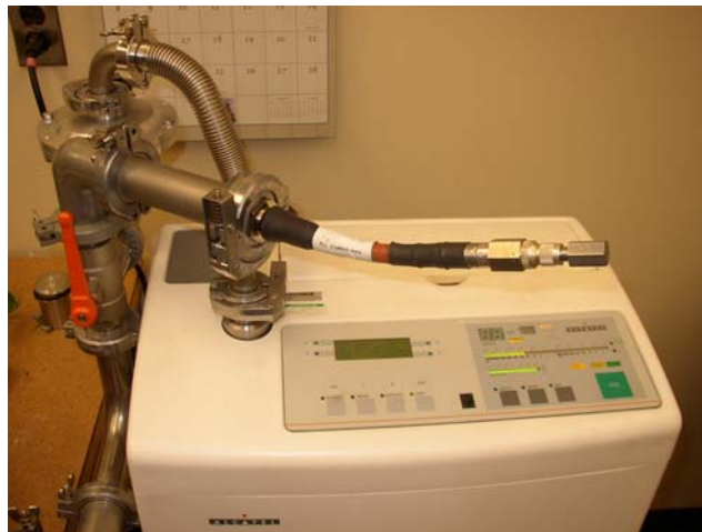
Figure 3 – Pressure Seal Test on Helium Leak Tester
