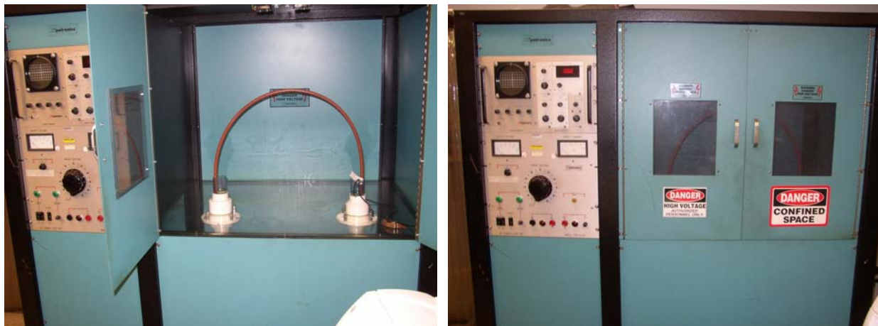
Figure 21 – Corona Extinction Test Setup
