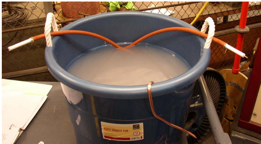
Figure 18 – Voltage Proof Immersion Test Setup
